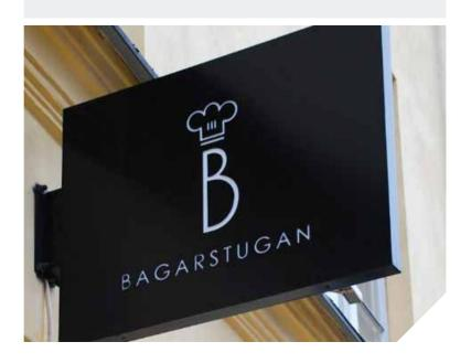
Light box in powder coated aluminum. White interior with LED. Front in 3 mm opal acrylic plastic with vinyl top. Powder coated aluminum frame screwed on to box sides. Boxes higher than 1000 mm are fitted with a hanging drop. Power supply hidden inside the box.
