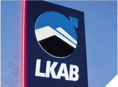
Light box in powder coated aluminum. White interior with LED. Front in 3 mm opal acrylic plastic. Powder coated aluminum front with milled decoration. Acrylic plastic attaches to aluminum front with 4 mm bolts, spacer and screw-nut. Front is attached to box. 10 mm acrylic plastic with or without vinyl top coating is glued to the 3 mm acrylic. Power supply hidden inside the box or placed in seperate transformer.
