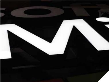
Channel letters with powder coated aluminum bottom. White interior with LED. 3 mm opal acrylic plastic front with vinyl top coating. Glued plastic ledge screwed to letter sides. Power supply hidden inside the letter.
