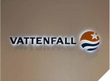
Backlit Channel letters with clear acrylic bottom, white aluminum middle with LED and top dimensional letter in powder coated aluminum. Front is screwed on to middle section. Studs for background distance. Power supply hidden inside the letter.
