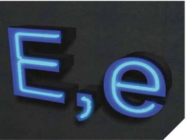
Dimensional letters in powder coated aluminium with front coaming to reduce light spill. Wire attached neon tubes. Transformer hidden inside letter.
