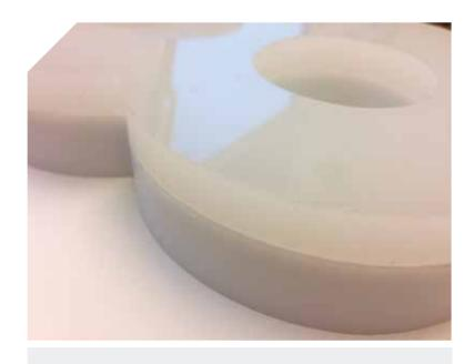
Channel letters with powder coated aluminum bottom. White interior with LED. Solid acrylic plastic front. Fronts screwed to letter bottom. Power supply hidden inside the letter or placed in seperate transformer.
