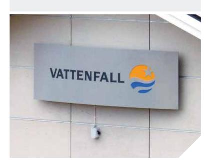
Light box in powder coated aluminum. White interior with LED. Front in 3 mm opal acrylic plastic with vinyl top. Powder coated aluminum front with milled decoration, with or without vinyl. Acrylic plastic attatches to aluminum front with 4 mm bolts, spacer and screw-nut. Front is attached to box. Power supply hidden inside the box.
