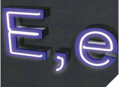
Dimensional letters in powder coated aluminium. Powder coated bottom, white aluminum middle with LED and top in powder coated aluminum with milled holes for LED. Front is screwed on to to letter sides. Power supply hidden inside the letter.
